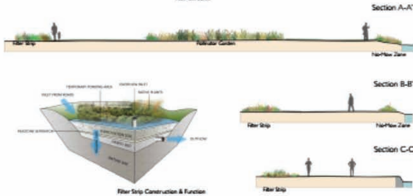
Filter Strip Construction & Function
